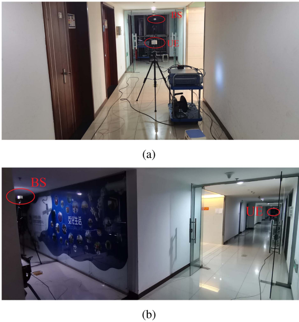
FIGURE 2. Measurement photographs taken in (a) the LoS scenario, and (b) the NLoS scenario.
