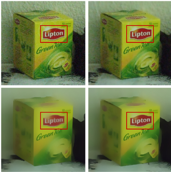
FIGURE 4. RGB denoising comparison between several strategies. Top-left: Noisy RGB image. Top-right: Guided by C_I . Bottom-left: Guided by Y_n . Bottom-right: Guided by Y_n + N_I .
