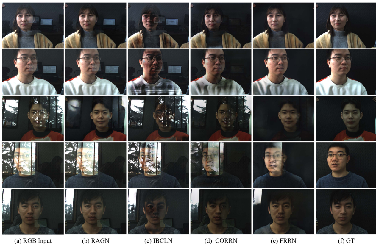
FIGURE 9. Visual quality comparison among FRRN and three state-of-the-art methods (RAGN [50], IBCLN [9], CORRN [51]) on the real dataset. FRRN successfully recovers the facial details in the regions occluded by reflections that are closest to the ground truth even in extremely harsh conditions.
