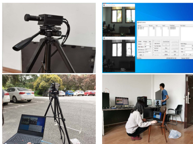
FIGURE 3. Top: JAI AD-130 GE camera and its graphical user interface (GUI). Bottom: Image capturing process using JAI AD-130 GE camera.
