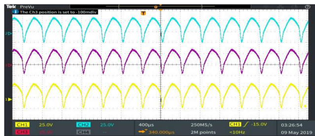
FIGURE 19. The experimental results corresponding to modular converter with three power modules: the three link voltages in each of the power module.
