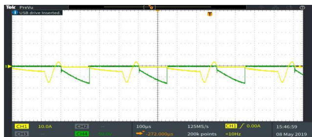
FIGURE 22. The experimental results corresponding to modular converter with three power modules: The voltage across the output-side switch, the current flowing through the output-side switch and its anti-parallel diode.
