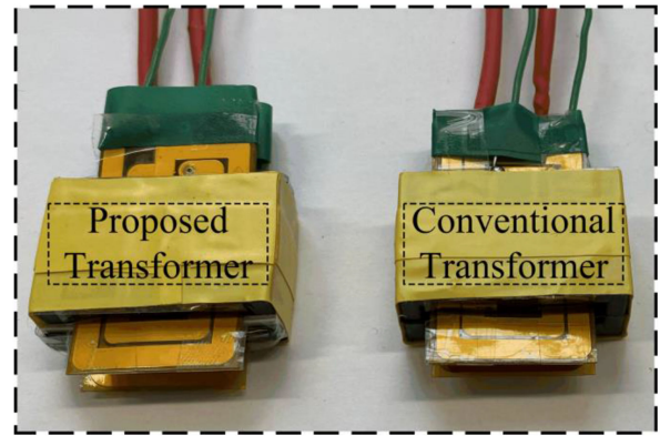
FIGURE 9. Prototypes of the proposed and inserted-segmental-shunt (conventional) topologies. Core: E32/6/20/R-3F4.
