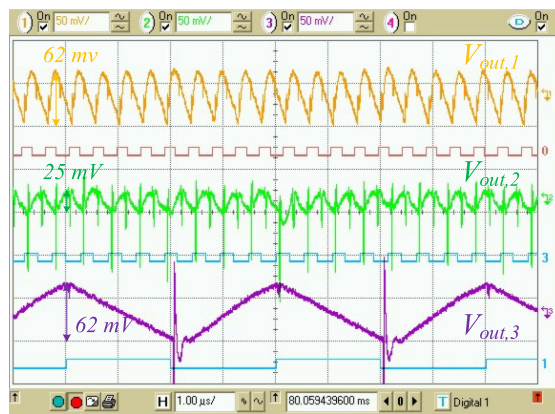
FIGURE 12. Experimental waveforms of the three SC converters. Ch.1 (yellow) (50 mV/div): Output voltage of the small area 75 mV output voltage ripple design. Ch.2 (green) (50 mV/div): Output voltage of the 25 mV output voltage ripple design. Ch.3 (purple) (50 mV/div): Output voltage of the high efficiency 75 mV output voltage ripple design. The digital signal D0 shows the control signal for low volume 75 mV design, D3 shows the control signal for the 25 mV design and D1 shows the control signal for the high efficiency 75 mV design.
