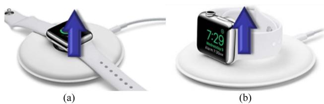
FIGURE 1. Current practice of wireless charging pad. (a) Fully aligned case. (b) When angular misalignment exists.
