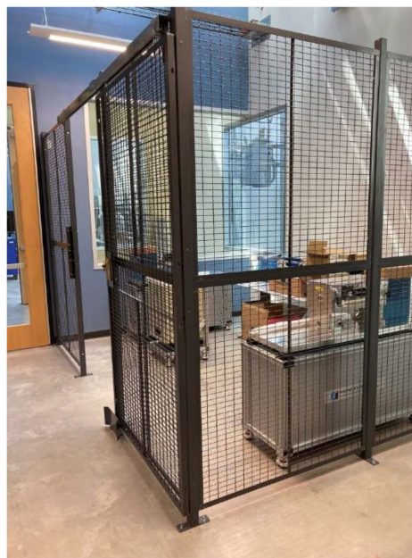
FIGURE 14. Protective barrier for testing up to 480 V and 60 A.
