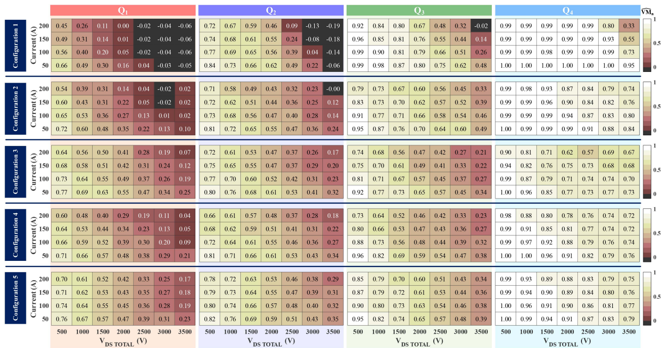
FIGURE 10. Normalized voltage margin for the different super-cascode configurations.
