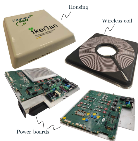
FIGURE 9. Low-profile battery charger based on FCI-DAB. Housing, coil and power boards.
