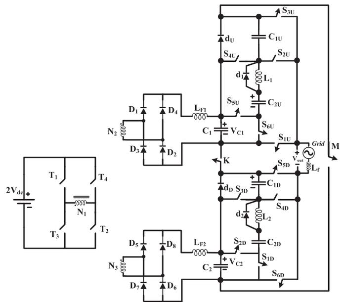
**FIGURE 6.** Modified grid-tied system for high power applications.
