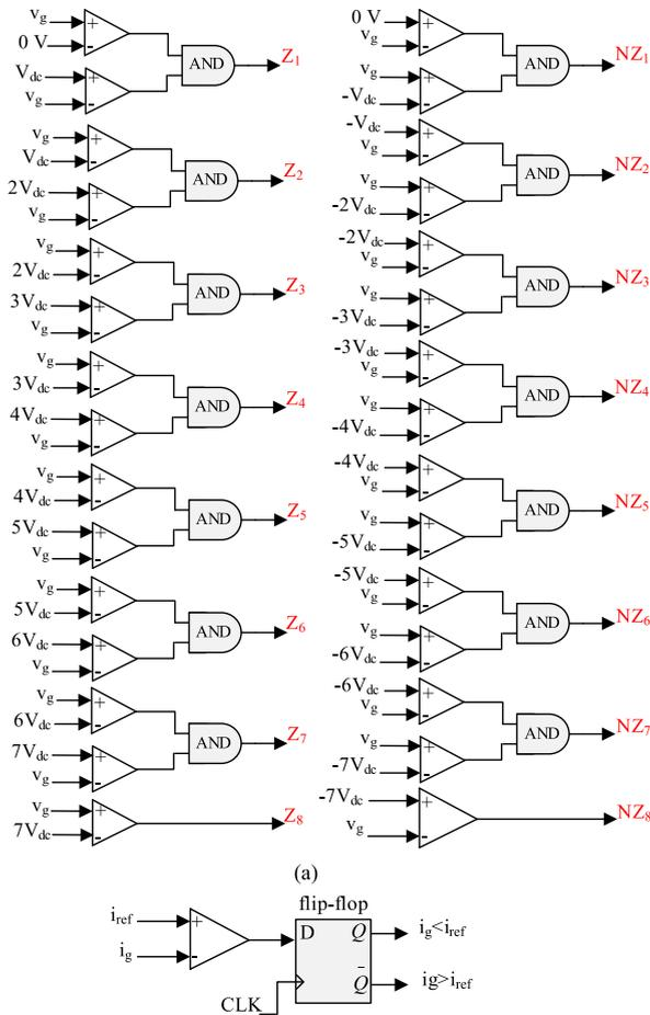
FIGURE 3. (a) Operation zones of modified inverter during positive and negative half-cycles, (b) voltage levels of the output voltage waveform during the positive and negative half cycle.
