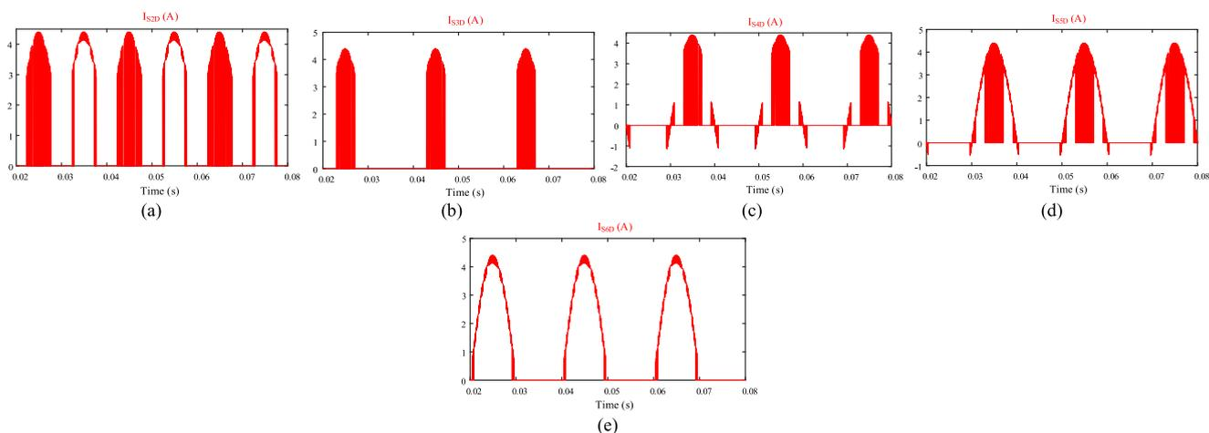
FIGURE 22. Simulation results: current stress of switches: (a) switch  $S_{2D}$ , (b) switch  $S_{3D}$ , (c) switch  $S_{4D}$ , (d) switch  $S_{5D}$ , (e) switch  $S_{6D}$ .
