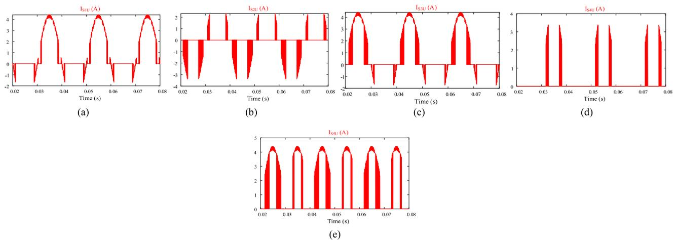
FIGURE 20. Simulation results: current stress of switches: (a) switch  $S_{1U}$ , (b) switch  $S_{2U}$ , (c) switch  $S_{3U}$ , (d) switch  $S_{4U}$ , (e) switch  $S_{5U}$ .
