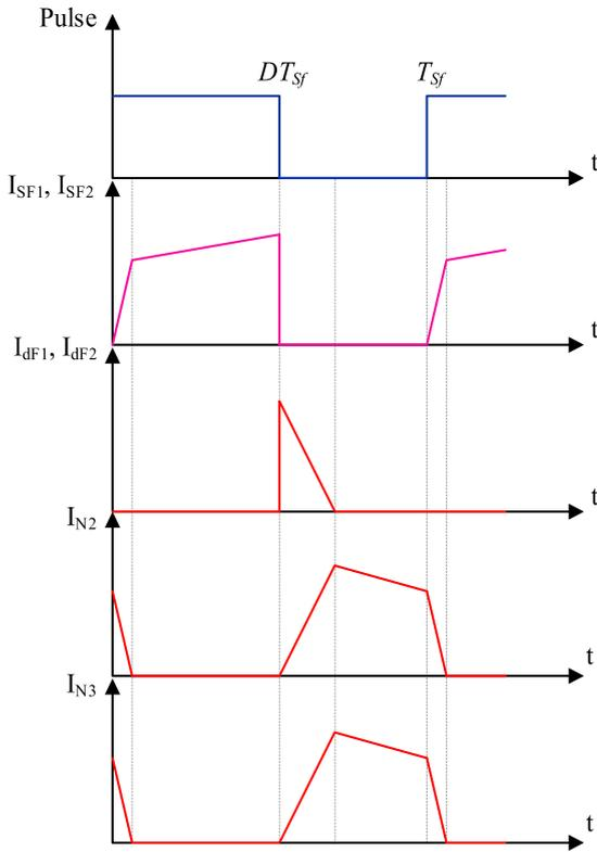
**FIGURE 5.** Switching states of the dual output flyback converter. (Note that,  $D$  and  $T_{sf}$  are the duty cycle and switching period of the flyback converter.)
