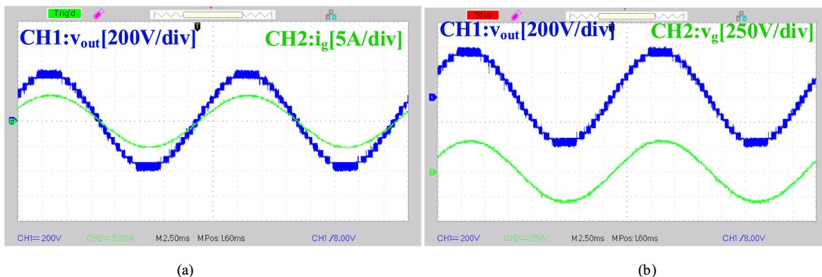
**FIGURE 27.** The experimental results: (a) the output voltage of the inverter (200 V/div) and the injected current (5 A/div) (b) and the local grid voltage (250 V/div) and injected current to the grid (5 A/div).
