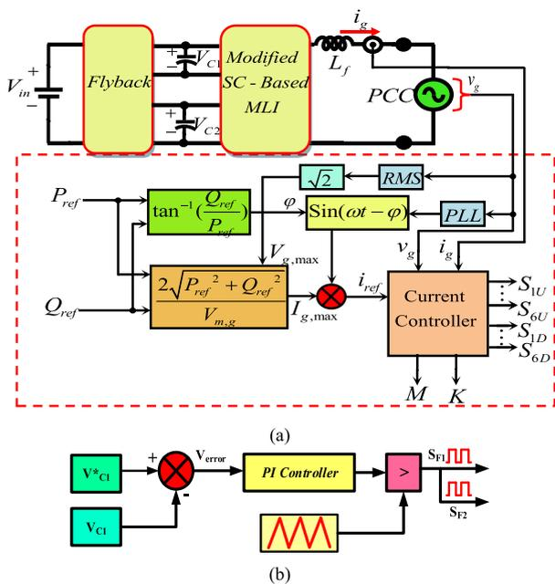
FIGURE 25. Schematic of control system applied for (a) modified SC-based MLI (b) fly back based DC-DC converter.
