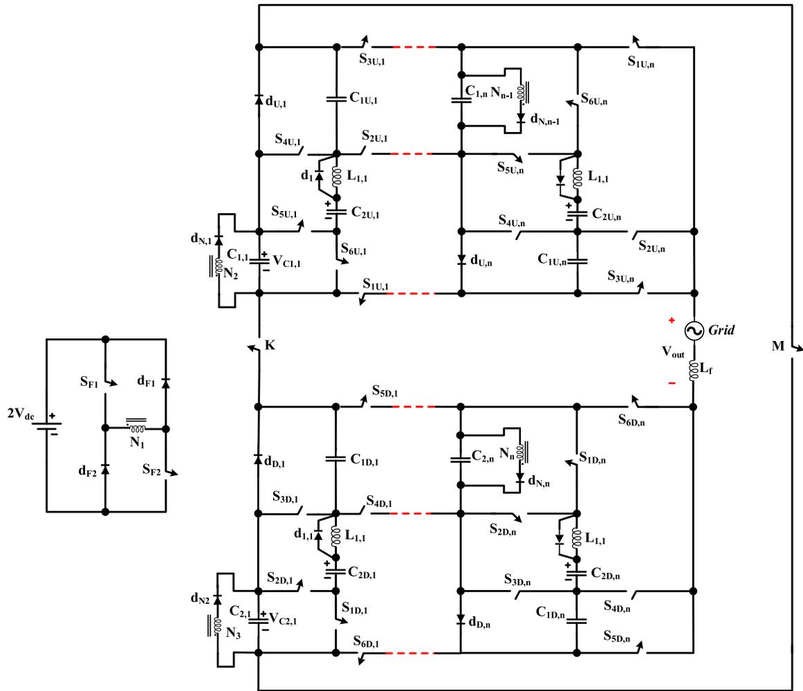
FIGURE 7. The extended version of the modified SC-based system.
