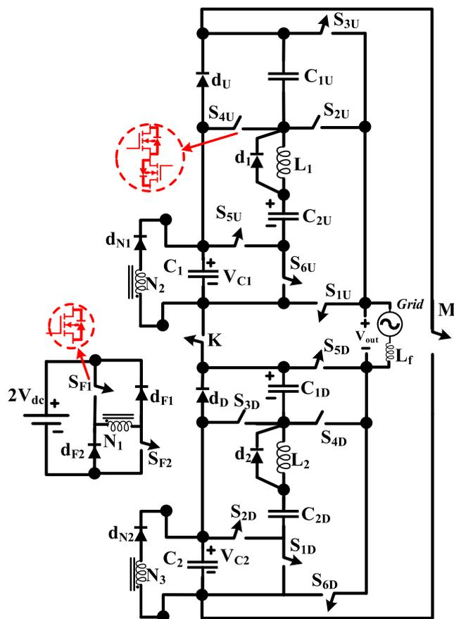
FIGURE 1. Modified grid-tied system.
