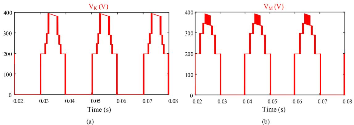
FIGURE 18. Simulation results: voltage stress of switches: (a) switch K, (b) switch M.
