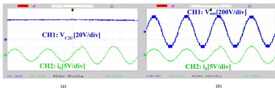
**FIGURE 30.** The experimental results under the applied step-change: (a) the voltage of the capacitor  $C_{2U}$  and the current of the grid (20V/div & 5 A/div) (b) the output voltage of the inverter and injected current to the grid (200 V/div & 5 A/div).
