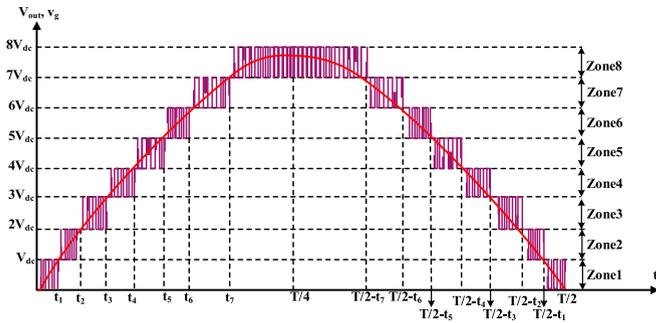
**FIGURE 2.** The output voltage waveform of the inverter, grid voltage, and eight operation zones of the modified inverter.
