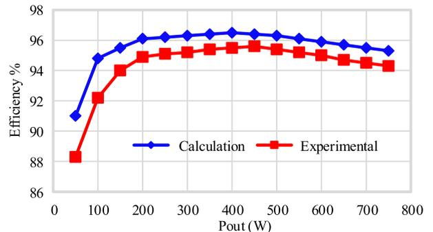
**FIGURE 11. The calculation and experimental efficiency curves of the modified inverter versus output power.**
