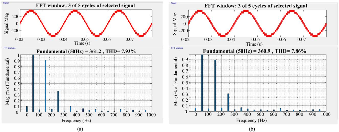
FIGURE 16. Simulation results: output voltage THD: (a) without using diode-inductor circuits, (b) with using diode-inductor circuits.
