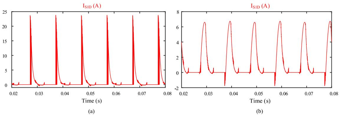
FIGURE 24. Simulation results: current stress of switch  $S_{1D}$ : (a) without using inductor  $L_2$  in charging path, (b) with using inductor  $L_2$  in charging path.
