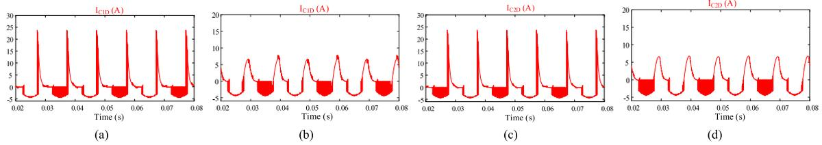
**FIGURE 13.** Simulation results: the current waveform of capacitor  $C_{1D}$ : (a) without inductor, (b) with an inductor, the current waveform of capacitor  $C_{2D}$ : (a) without inductor, (b) with an inductor.
