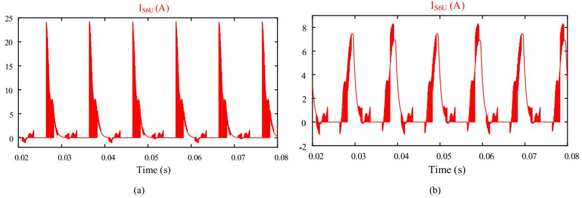
FIGURE 23. Simulation results: current stress of switch  $S_{6U}$ : (a) without using inductor  $L_1$  in charging path, (b) with using inductor  $L_1$  in charging path.
