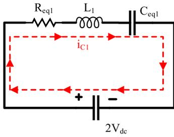
**FIGURE 8.** The equivalent circuit of capacitors  $C_{1U}$  and  $C_{2U}$  charging loop.
