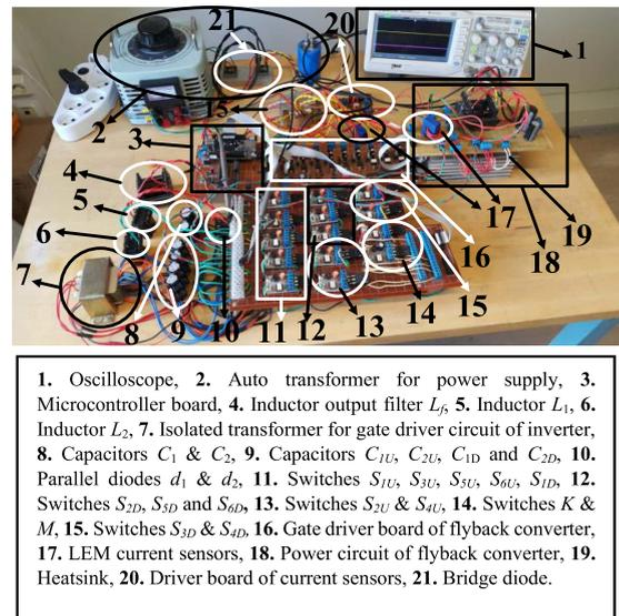
FIGURE 26. Photo of the experimental prototype of the modified topology.
