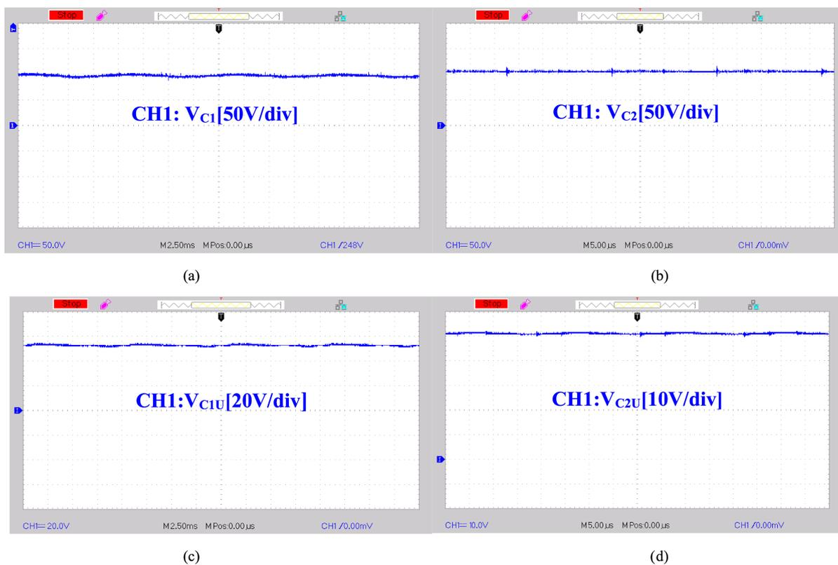
**FIGURE 28.** Voltage across (a) the capacitor  $C_1$  (50 V/div) (b) the capacitor  $C_2$  (50 V/div) (c) the capacitor  $C_{1U}$  (20V/div) (d) the capacitor  $C_{2U}$  (10V/div).
