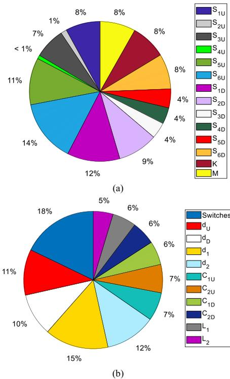
**FIGURE 10. (a) Pie chart of the inverters’ power switches distribution, (b) pie chart of the inverters’ total switches power losses, diodes, capacitors, and inductors distributions.**
