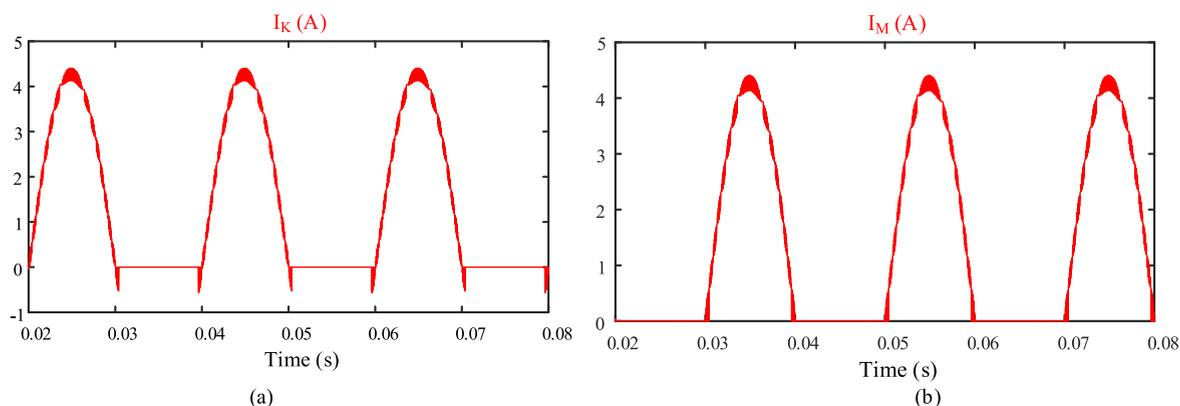
FIGURE 21. Simulation results: current stress of switches: (a) switch K, (b) switch M.
