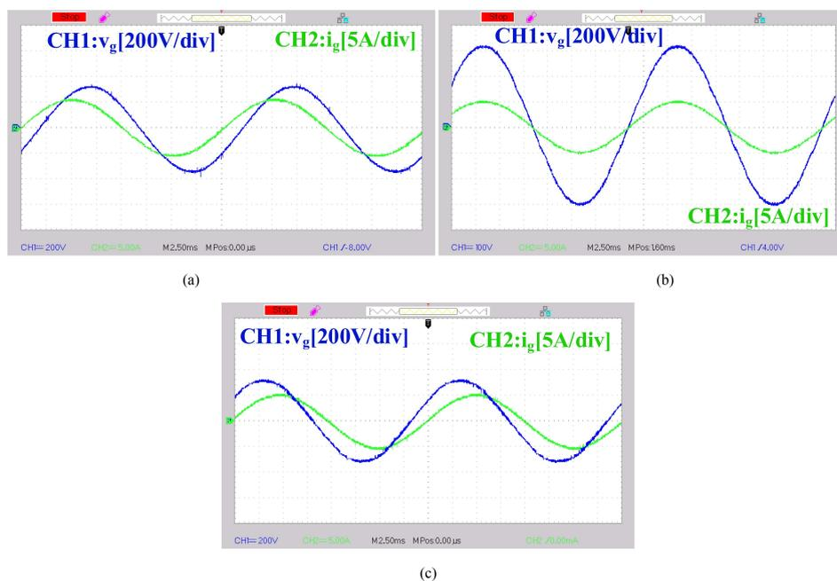
**FIGURE 29.** The grid voltage and the injected current waveforms under: (a) leading PF (200 V/div & 5 A/div) (b) unity PF (100 V/div & 5 A/div) (c) lagging PF (200 V/div & 5 A/div).
