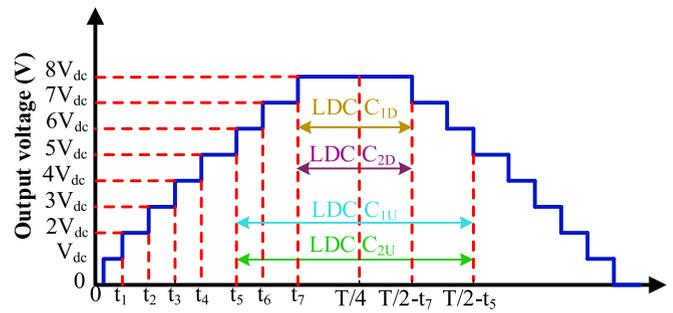
FIGURE 9. The typical output voltage waveform of the modified MLI inverter during positive half-cycle.
