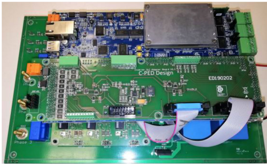
FIGURE 16. Three-phase PFC prototype based on a Hybrid Module.
