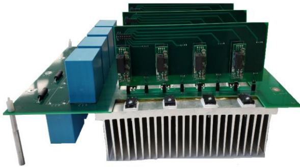
FIGURE 12. Experimental prototype picture of a 20-kW hybrid Si/SiC switch based ANPC inverter.
