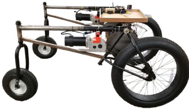
FIGURE 1. Rx Robotics autonomous horticultural rover, the ‘bikebot’. The rover is currently an electrically powered wheeled vehicle, which will be remodeled with tracks.
