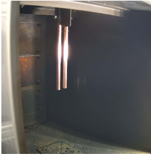
FIGURE 4. EPRI enclosure with vertical copper electrodes.
