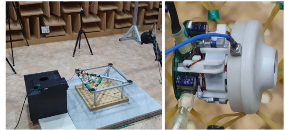
FIGURE 14. Noise and vibration measurement apparatus.
