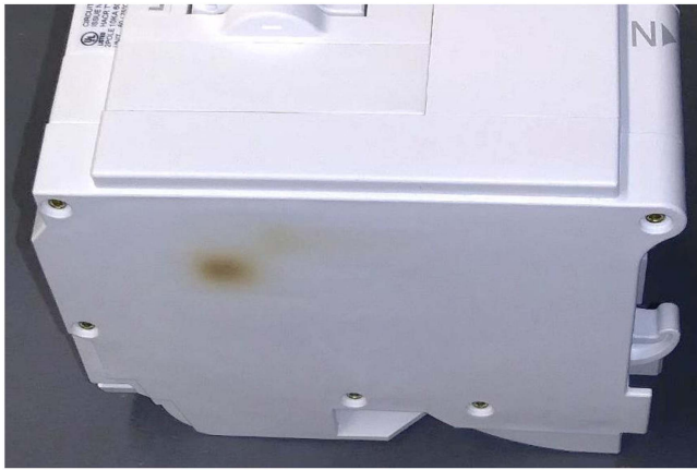
FIGURE 9. Scorched area on this defective brand 14 20 A H-M type breaker developed before it finally tripped at 59 A (296% of rated current).
