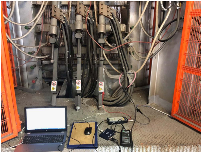
FIGURE 15. Instrumentation connected to the electrodes: measurement of the current circulating in a single electrode.
