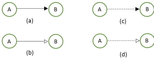
FIGURE 5. Bond graph modeling of: (a) data flow, (b) command signal, (c) data flow with protected channel and (d) command signal with protected channel.
