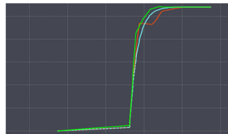
FIGURE 12. Cylinder with PID control. Ideal (blue), distributed with random delay(red), distributed with TAC (green).
