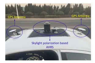
FIGURE 8. Vehicle test.
