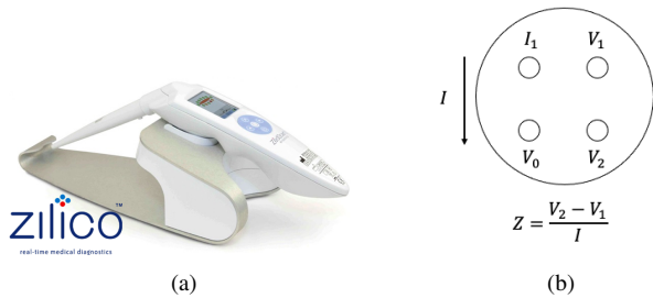
Fig. 1. Electrical Impedance Spectroscopy device: (a) ZedScan™ [12], (b) tip of the tetrapolar probe showing the principle of the measurement, a known current I flows between the active electrodes ( I_1 and V_0 ) while the passive electrodes ( V_1 and V_2 ) capture the potential difference at each frequency
