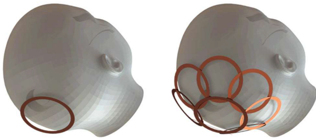
Fig. 1. Renderings of typical single-element (left) and array coil (right) setups. RF array coils are commonly comprised of multiple (often but not necessarily overlapped) loop elements conformed to the anatomy of interest to retain the benefits of small loop coils over an extended field-of-view.
