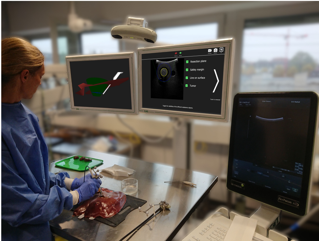
Fig. 1. The navigation system in a demo setup with the optical tracking camera, the navigation screens, the navigated instruments and the operator.
