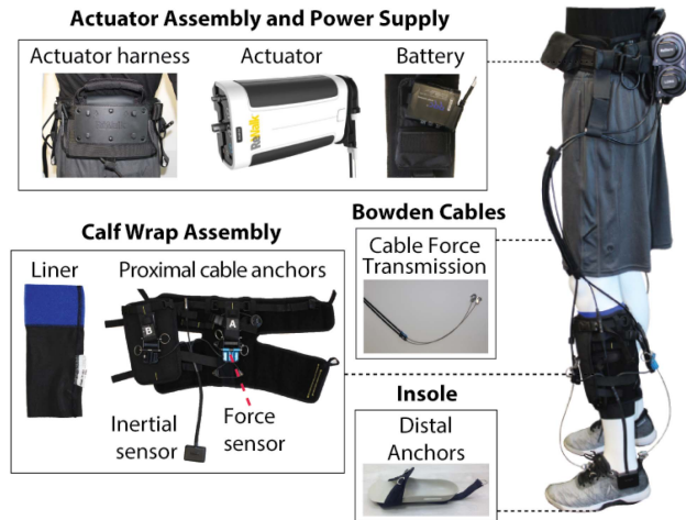
FIGURE 1. Soft Robotic Exosuit, ReWalk ReStore suit components. The ReStore is a textile-based exosuit that provides mechanical assistance to the paretic plantarflexors and dorsiflexors during walking.
