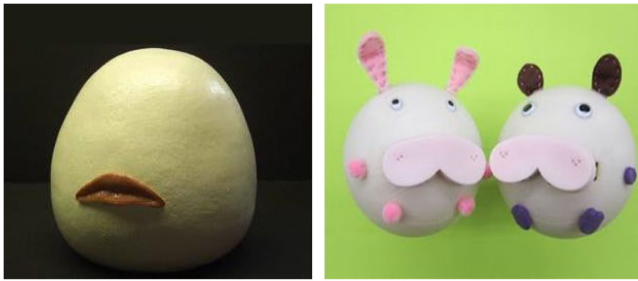
FIGURE 3. Left: first version of Kissenger was a head-shaped device with a realistic pair of lips. Right: second version of Kissenger was designed to look like a cute animal character with soft silicone lips.
