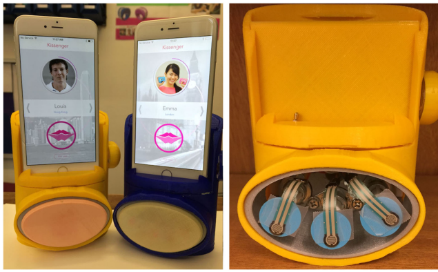
FIGURE 6. Left: A pair of prototypes of the Kissenger device was designed and implemented with iPhone 6 Plus. Right: The force sensors and linear actuators beneath the flexible lip cover.
