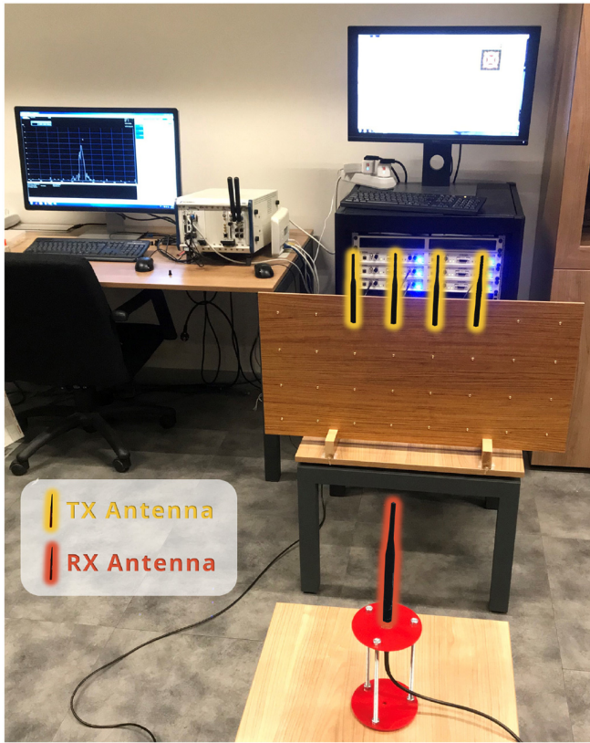
FIGURE 4. 4 × 1 test-bed which performs antenna selection at the transmitter.
