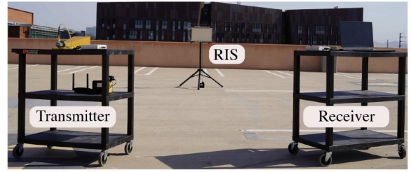
FIGURE 15. The RIS-assisted wireless communication system consists of an RIS, a transmitter (BS), and a receiver (UE). The transmitter and receiver are portable and can be placed in the far-field of the RIS surface.
