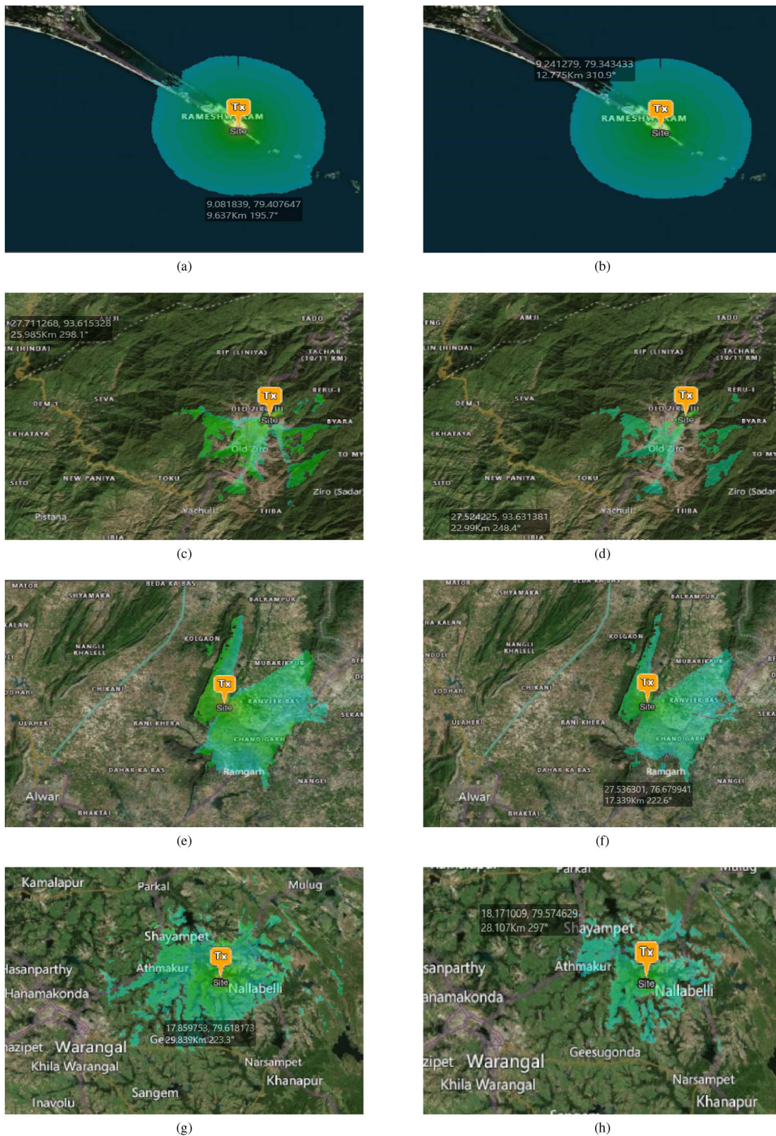
FIGURE 12. Coverage plots with 10 m antenna height at I - 700 MHz with bandwidth of 5 MHz and II -3800 MHz with bandwidth of 10 MHz: Dhanushkodi (I (a), II (b)), Lempia (I (c), II (d)), Bandholi (I (e), II (f)) and Muddunoor (I (g), II (h)).
