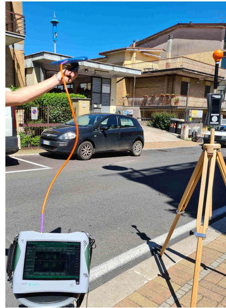
FIGURE 3. Example of parallelization of task T4 (right - EMF meter) and tasks T1-T3 (left - portable SA) in a measurement location.
