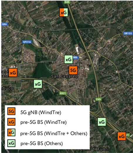
FIGURE 4. Output of Phase 1 - deployment characterization in an area of around 12.4 [km 2 ], centered over the town of San Cesario (Italy). The figure reports positioning, supported technologies (including or not 5G equipment), hosted operators (WindTre, Others, WindTre + Others) of each base station over the territory. One base station located in the town center provides 5G services for the WindTre operator.
