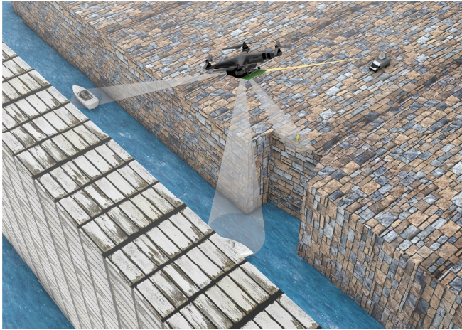
FIGURE 1. UAV equipped with a lightweight RIS covering first-responder team and victims in an emergency scenario.
