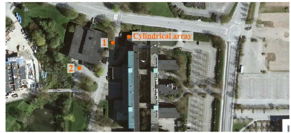
FIGURE 2. The outdoor scenario for both LOS (position 1) and NLOS (position 2). The base station has a cylindrical array and is positioned on the roof. The users were moving within a circle with a diameter of 5 m.
