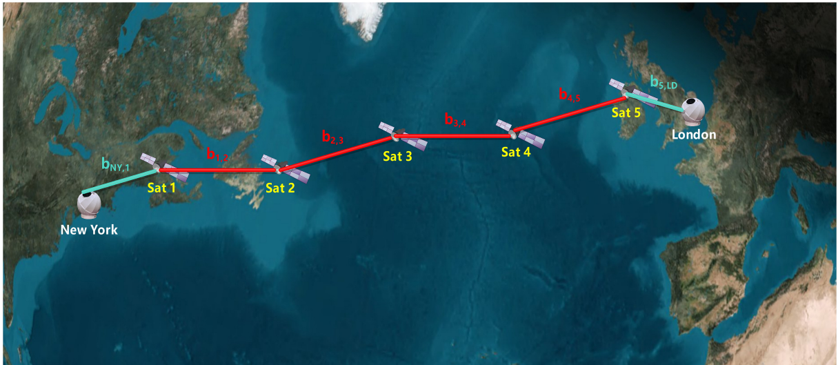
FIGURE 2. An illustration of the transmission power of each link on the path for the inter-continental connection from New York to London.
