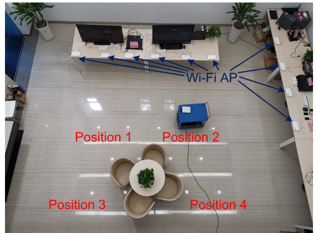
FIGURE 12. An illustration of the experimental setup with four receiver locations.
