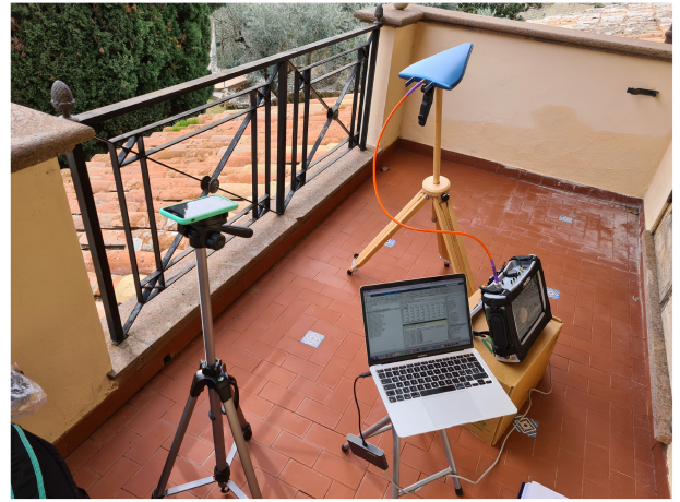
FIGURE 7. Positioning of traffic chain (smartphone and tripod) and SAN chain (SAN, directive antenna, tripod, control laptop and cables) during ATA assessment.
