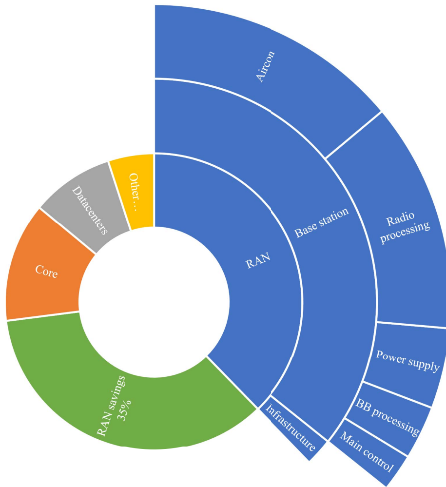
FIGURE 15. The energy consumption of the mobile network in the inner circle, showing 48% energy consumption savings in the RAN, corresponding to 35% of the total mobile network energy consumption. The middle circle shows the share of the RAN, divided out on base stations and infrastructure. The outer circle shows the base station components.
