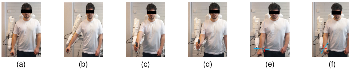
Fig. 4. Experiment steps for the first part of performance evaluation (a) initial configuration, actuation of (b) second, (c) third, (d) fourth, (e) sixth, and (f) last joint. The joints in actuation work in trajectory tracking mode, while others are in set point control mode.
