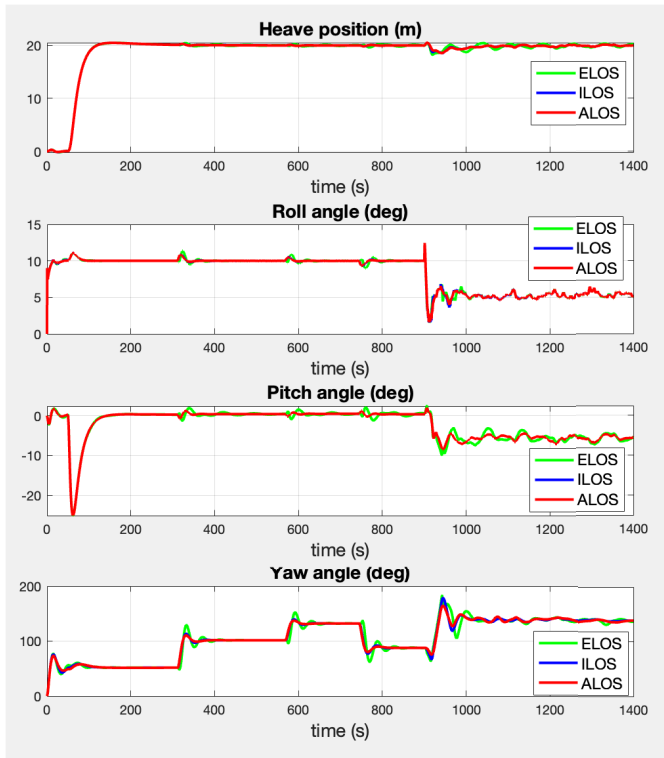
Fig. 6. Depth z^n (m), roll angle \phi (deg), pitch angle \theta (deg), and yaw angle \psi (deg) for the ELOS, ILOS, and ALOS guidance laws.
