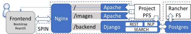
Fig. 8: ScienceSearch deployed in NERSC’s Spin. Docker containers (round blue boxes) can access internal (rancher fs) and external HPC (project) storage.
