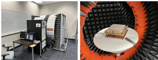
FIGURE 15. Testing of the fabricated TCDA prototype within our MVG Starlab anechoic antenna chamber from 650 MHz to 5.85 GHz.
