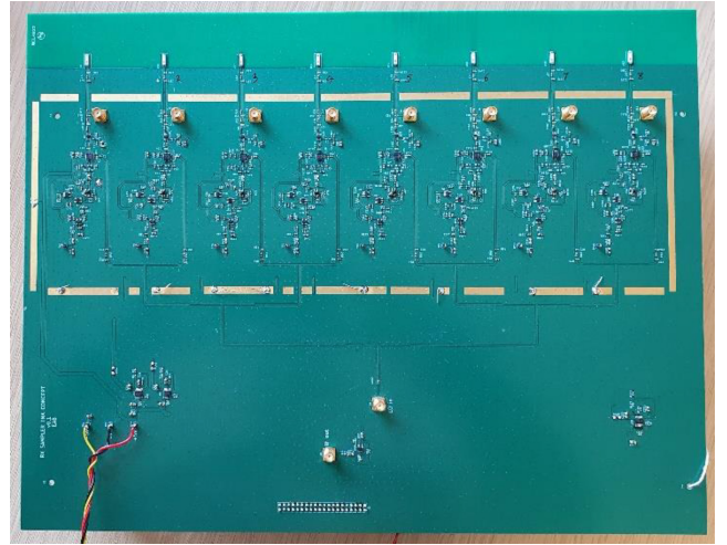
FIGURE 12. Built PCB showing 8 STMA RX cells (antennas and test connector for cell calibration visible at top, IF2 output and LO input connectors towards bottom).
