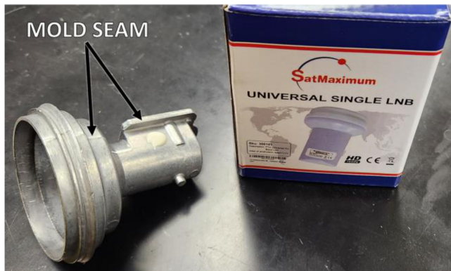
FIGURE 1. Commercial off-the-shelf metal cast, aperture matched corrugated conical horn, with mold seam annotated.
