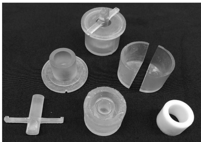
FIGURE 4. The PDMS negative mold, and both assembled and disassembled positive molds 3D printed from BioMed Clear resin.
