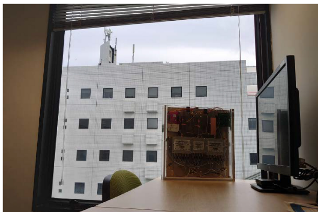
FIGURE 11. Field test measurement of the multi-band dual-polarized ambient RF powered wireless sensor inside the computer barn in the HKUST campus at location L5 (see Figure 1). The base station (outside window at top left) is approximately 50 m away and our system is seen in the bottom right silhouetted in the foreground of the window. The system was entirely powered by the ambient RF cellular signals in the environment.
