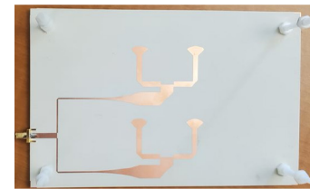
FIGURE 22. (a) Schematic view of the 2x2 CSAA prototype, (b) feeding network of the prototype, (c) fabricated top view of the 2x2 CSAA prototype, and (d) fabricated bottom view of the feeding network. The feeding network has three T-Junctions, tapered transmission lines, and radial stubs.
