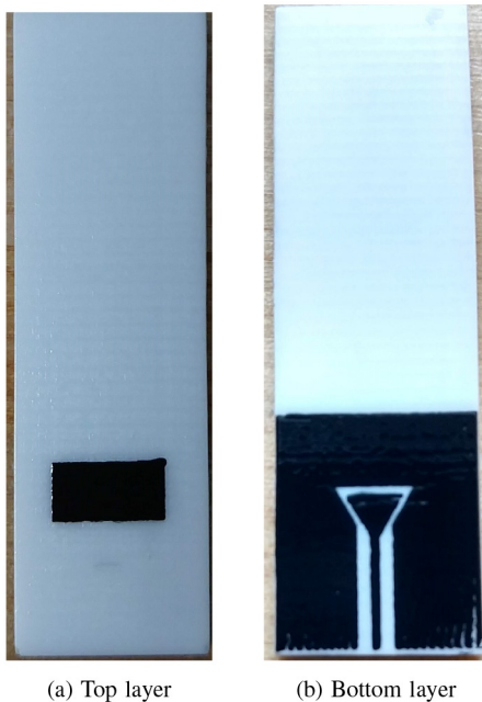
FIGURE 11. Micro-dispensed platinum ink on the 3D-printed YSZ substrate before drying process.
