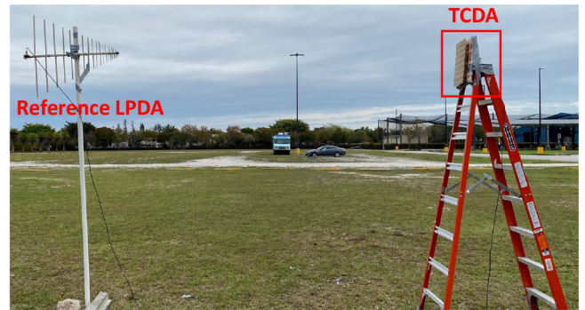
FIGURE 19. Far-field gain measurement set up with a high gain LPDA as the reference antenna.
