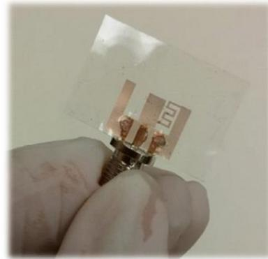
**FIGURE 8.** Flexible and transparent frequency reconfigurable mesh antenna. (Reproduced from [42] with permission. Copyright © 2017 IEEE).
