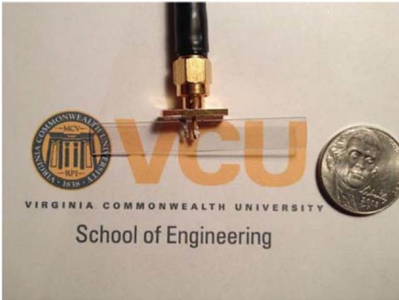
**FIGURE 28.** Fabricated transparent GZO dipole antenna. (Reproduced from [9] with permission. Copyright © 2017 Wiley Periodicals, Inc).
