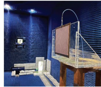
FIGURE 8. (a) Photographs of the fabricated array antenna and (b) measurement setup.
