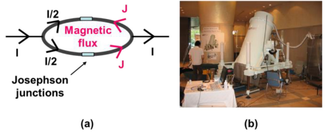
FIGURE 2. (a) Operation principle of a typical SQUID. (b) A SQUID system in superconducting magnetic shield [58].
