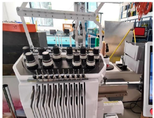
FIGURE 1. Specialist digital embroidery machine at Loughborough University for embroidering conductive threads. The designs can be converted into a picture and then fabricated automatically. It is important to be able to control the machine tensions as the threads are designed for their conductivities not their physical properties. The machine can also control the stitch spacing and direction.
